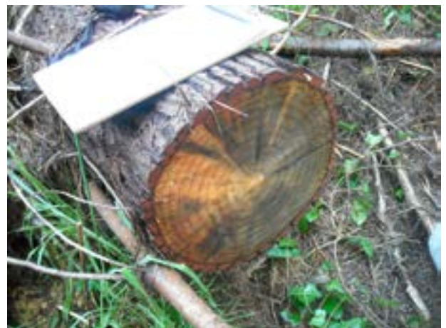
Severe sapstain in a tree felled during a storm in a Pinus radiata plantation.
