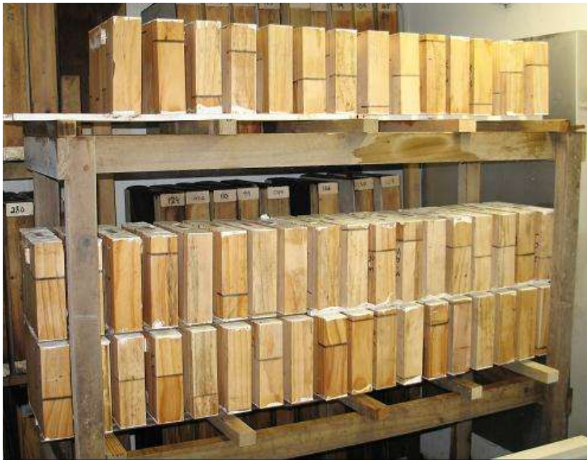
Figure 1: – Sample blocks in a temperature and humidity controlled conditioning room
