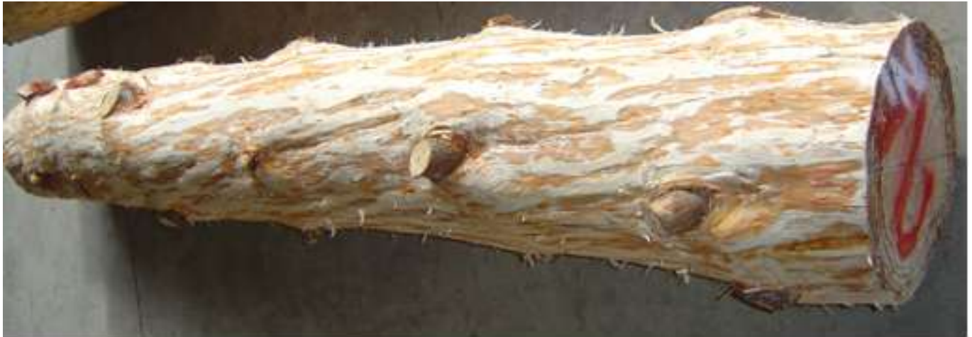
Figure 1: Radiata log with severe left-hand (S) spiral grain
