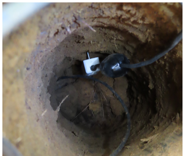
Soil moisture sensor installed at a Forest Flows site.
