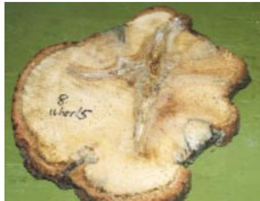
Radiata pine whorl section demonstrating typical stain and decay
