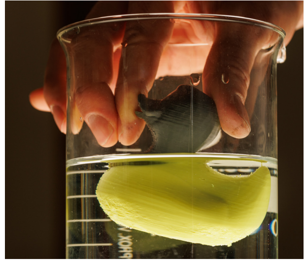
A colour-changing and flexible 4D printing filament developed by Scion.
