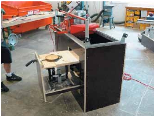
Figure 1: Discs are placed on an adjustable height table and inserted into the housing. The saw then passes over the samples.
