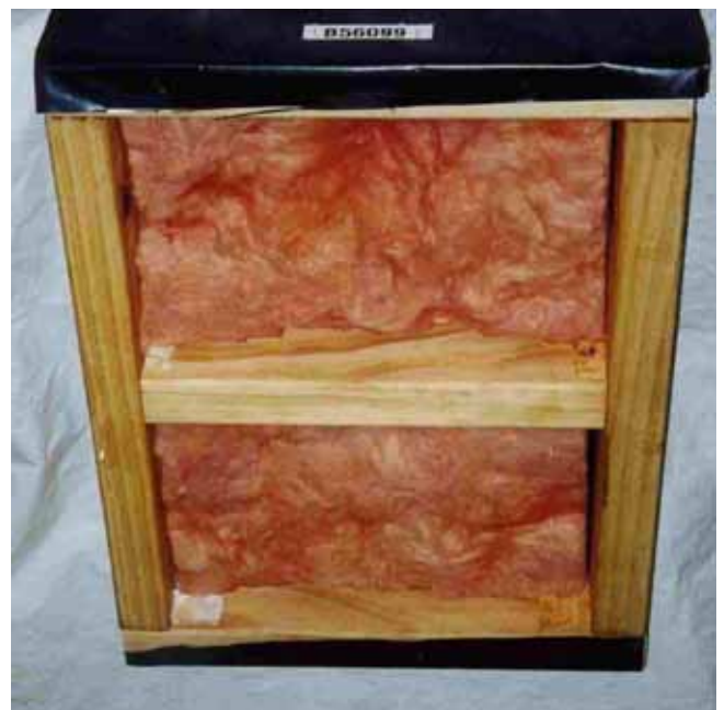
Figure 1: Frame unit with inoculation strips attached left and right on dwangs and bottom plates, before enclosure with building paper and fibre-cement cover.
