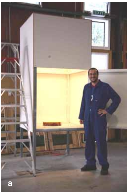
Figure 3: (a) Photo Booth with controlled light and camera function. (b) Photo Image illustrating fine detail of growth rings and pathological heartwood.
