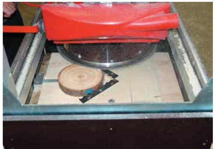
Figure 1: Discs are placed on an adjustable height table and inserted into the housing. The saw then passes over the samples.
