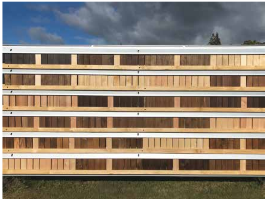
In 2021, a field test was set up at Scion's Rotorua campus to test flat panel durability of the heartwood of Cupressus lusitanica, C. ovensii and Douglas-fir with and without heat modification (at 230°C) along with a number of control samples.
