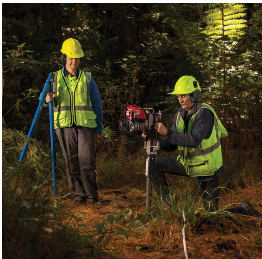
Soil percussion auger - taking an intact soil core down to one metre, which tells us the nutrient stocks on site in the soil.
